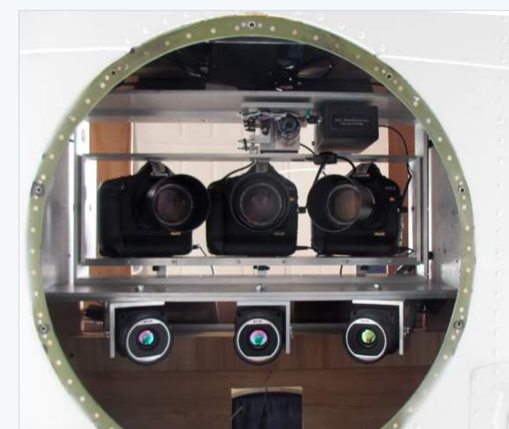
Three Canon EOS-1Ds Mark III's (top) paired with three FLIR SC645 thermal sensors in the belly-port of a Twin Otter. The left and right instruments are angled to avoid overlap.
